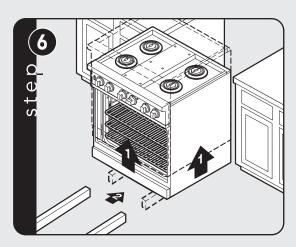
Lift unit and prop on wood blocks.
